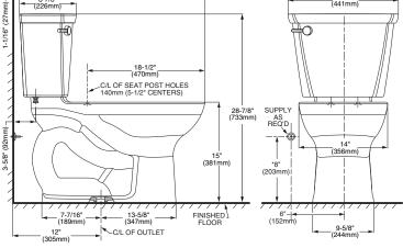
THIS TOILET IS DESIGNED TO ROUGH-IN AT A MINIMUM DIMENSION OF 305MM (12") FROM FINISHED WALL TO C/L OF OUTLET.
