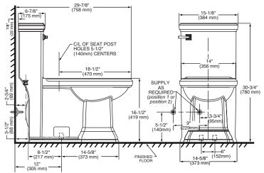
IMPORTANT: Water supply on the wall is required at 3-3/4" or 9" from centerline of the toilet (see rough-in). First suggested position is hidden behind the toilet. The geometry of the toilet gives space for this installation. The second suggested position is next to the toilet. Between these two positions, the space for the supply between wall and toilet is limited to 3-1/4". In this case, check your supply and hose dimensions
