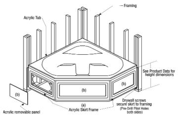
\*Note: To prevent the skirt from flexing, mount a back support (1'x3" approximately) horizontally and centered directly behind the skirt.
