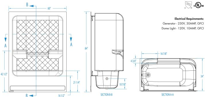
FEATURES Ibs (kg) Dimensional Tolerance ± 3/8". Dimensions needed for site preparation should be measured from the unit. Aquatic assumes no responsibility for preparatory work.
