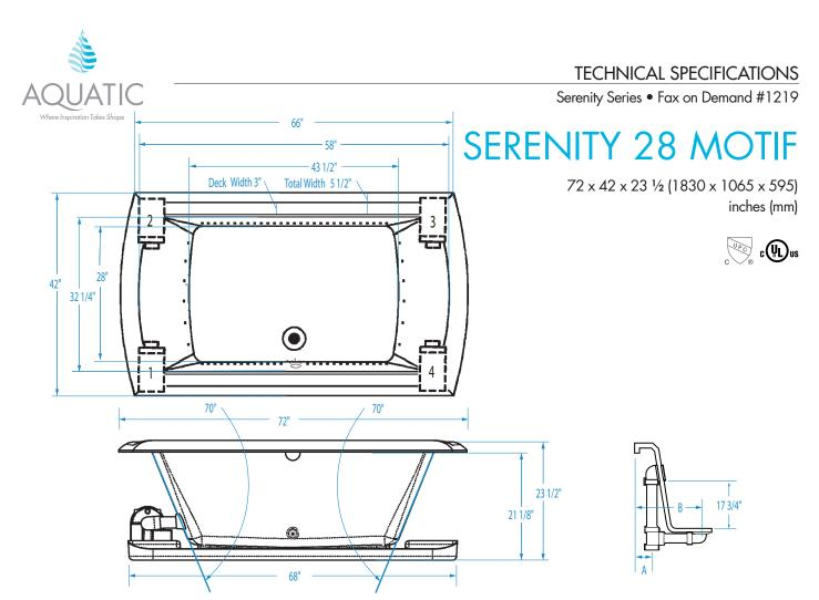
FEATURES Ibs (kg) Dimensional Tolerance ± 3/8". Dimensions needed for site preparation should be measured from the unit. Aquatic assumes no responsibility for preparatory work.
