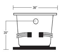
FEATURES | lbs (kg) | Dimensional Tolerance ± 3/8". Dimensions needed for site preparation should be measured from the unit. Aquatic assumes no responsibility for preparatory work.
