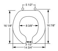
Ring thickness is 13/16" Ring thickness including the bumper is 1-1/16" Height of the seat with cover is 2-5/16"
