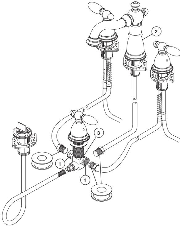
From tub valves, connect hot and cold water lines to labeled inlets (1) on transfer valve. Either inlet (1) may be used for hot and cold. Use plumber tape on threaded connections. Connect tub spout (2) to remaining outlet port (3) on transfer valve. **WARNING: Excessive heat during installation may damage internal components. Removal of the diverter is recommended prior to installation if excessive heat will be used.**
