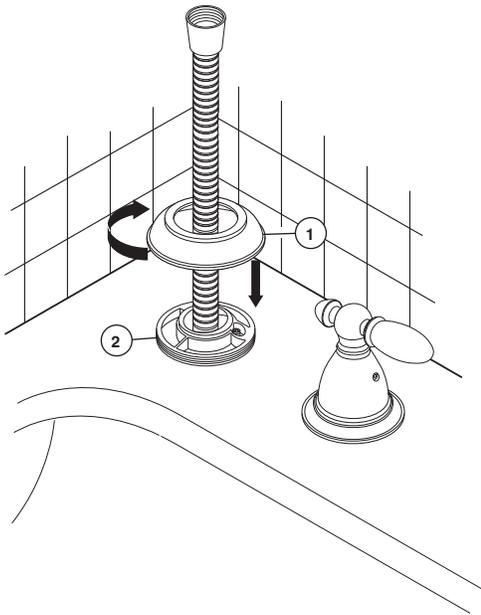
**C.** Install base (1) to nest (2) and tighten. **OPTION: Use silicone under the base if deck is uneven.**
