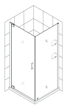
43. Mark the **Glass shelf (22)** position on the wall. According to the measurements in Fig. 46.1, mark the drilling holes for the **Shelf brackets (without nut) (31)**. Drill the holes using Ø **5/16**" drill bit and insert the **Wall anchors (23)**.
