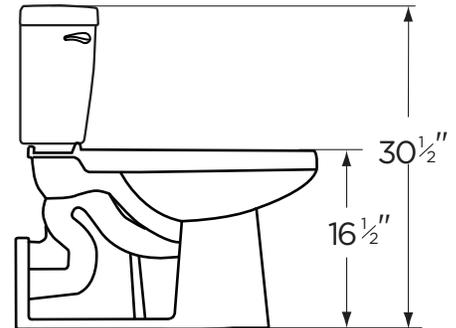
THIS FIXTURE QUALIFIES ACCORDING TO ASME TEST PROCEDURES AS A LOW CONSUMPTION WATER CLOSET WITH AN AVERAGE CONSUMPTION OF 1.6 gpf (6.0 Lpf) OR LESS.
