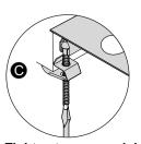
Tighten to secure sink.
