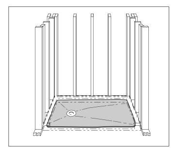
4. With the stainless steel clips installed on the threshold, place the barrier-free shower floor into the framework and firmly press it into the mortar/thinset. The outer perimeter of the shower floor should contact the subfloor.
