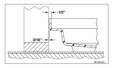
After the shower floor installation is complete, install 1/2" moisture-resistant wall board, as shown. The ideal installation results when the outside surface of the wall board and shower floor flange are flush, as shown in the illustration below.
