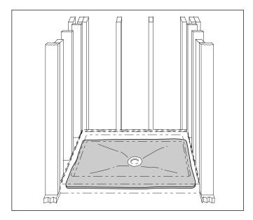
Place the shower floor into the rough opening and firmly press it into the mortar/thinset. The exposed front bottom edge(s) of the shower floor should contact the subfloor.
