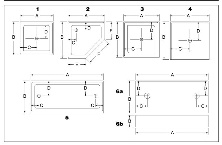
These dimensions are approximate sizes only. For proper fit, measure the actual shower floor prior to building the framework to determine the exact size. Add 3/8" to the width measurement and at least 3/16" to the depth measurement of the actual shower floor to create the size of the framework opening needed.
