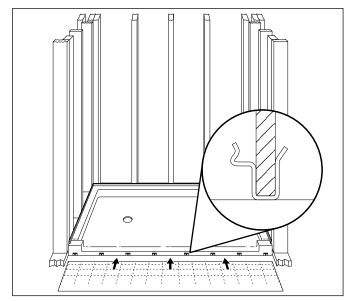
3. Place up to a 1/2" thick layer of mortar/thinset on the floor. This will ensure complete contact and support by the existing subfloor, eliminating shower floor flex during normal use. Taper the mortar/thinset to 1/4" thick around the floor drain. Mix enough material to cover the area under the shower floor. Do not place the material closer than 2" to the edge of the shower floor or the drain opening.
