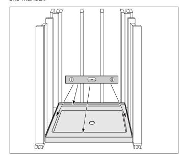
**Note**: The ideal installation results when the outside surface of the wall board and shower floor flange are flush, as shown in the illustration below. This dimension allows the Swan wall panels or alternate shower wall material, to rest against the lip of the shower floor once the moisture-resistant wall board is installed, as shown in the second illustration below.
