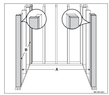
3b. For existing construction, dry fit the shower floor to make sure it fits correctly in the shower enclosure framework. If necessary, modify the framework to achieve the proper shower floor fit. The illustration below shows the ideal shower floor flange to existing wall surface gap of 3/16"
