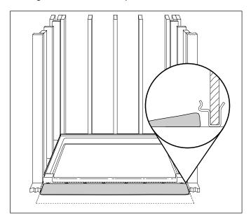
**Note**: The barrier-free shower floor ramp can be installed on the same floor surface as the shower floor or can be installed on raised floor surface (up to 1/2" thick), as shown below.
