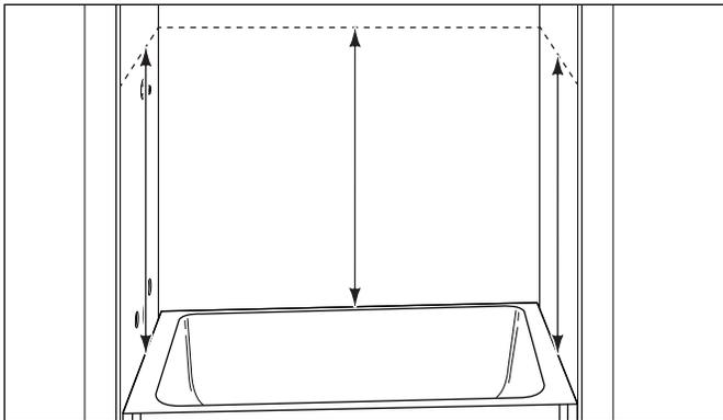
3. Transfer these measurements to both side panels and the back panel. Cut the bottoms of the panels.
