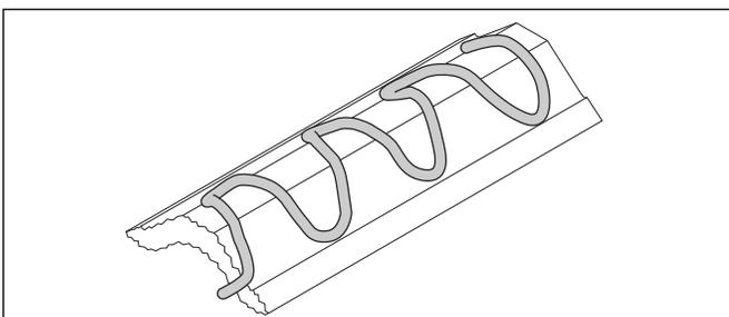
5. Press the corner moldings into place. Remove any excess silicone.
