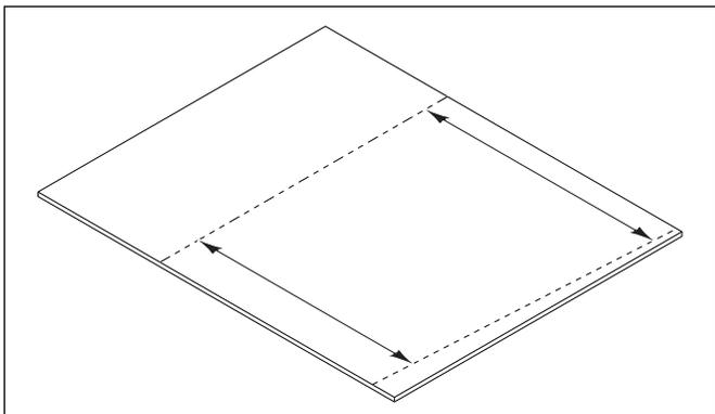
**Note:** On subway tile and square tile panels, this process will keep the faux grout lines running level, although the bottom tiles may not be evenly sized from the tub to the first faux grout line. Since every installation is slightly different, it is up to the installer to create a pattern match that is visually pleasing.
