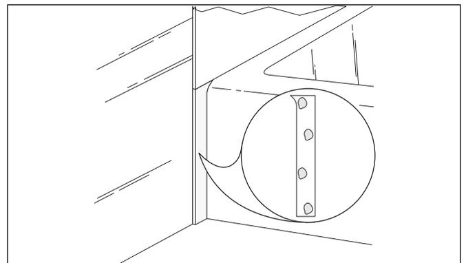
**Note:** Make sure the top edges of both apron strips are against the bottom lip of the side panels.
