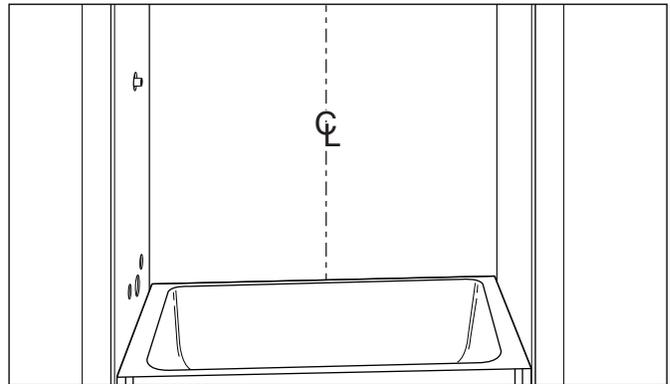
6. Take several measurements, bottom to top, from the center line to each wall surface. These measurements will ensure the back panel fits the exact contour of the two side walls.
