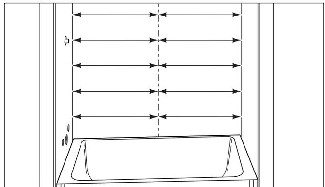
6. Place the panel, finished side facing up, on a flat surface. Using a pencil, lightly mark the center of the back panel.
