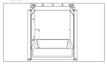
After marking the height, draw a 4 inch level line on both walls. These lines will be used to align the top edges of the soap dish.
