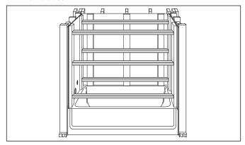
Insert (wedge) blocks or cross braces between the front to rear panel braces and the back panel braces. These blocks or braces must apply pressure to the back panel to hold it in place.
