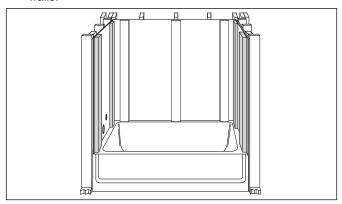
Install (wedge) horizontal braces against the left and right wall braces.
