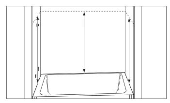
Transfer these measurements to both side panels and the back panel. Cut the bottoms of the panels.
