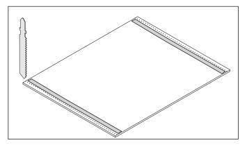
Dry fit the back panel, and make any necessary adjustments. Temporarily secure the back panel to the wall in order to properly fit the side panels.
