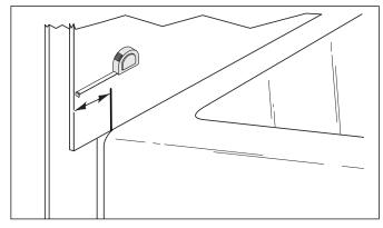
Hold the apron strips in place and scribe the angle of the bathtub base onto each piece. Remember, do not cut the finished edge.
