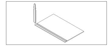
5. Dry fit the panel, and make any necessary adjustments.
