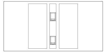
a. Select any one of the four flat panels for positioning on the back wall. Apply adhesive to the back of the panel, keeping the adhesive at least one inch from the panel edges.
