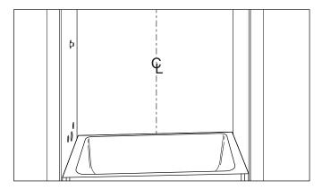
Take several measurements, bottom to top, from the center line to each wall surface. These measurements will ensure the back panel fits the exact contour of the two side walls.
