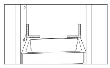
2. If the tub surface is not perpendicular to the wall, use a level and draw a line around the alcove on all three walls. Measure the distance from the line to the top of the tub.
