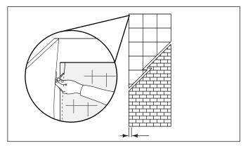
Place the wall panel, finished side facing up, on a flat surface. Place pieces of masking tape over the area where the saw contacts the Swanstone panel.
