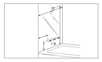
6. Transfer the measurements to the panel.
