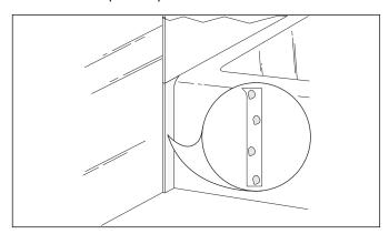
**Note**: Make sure the top edges of both apron strips are against the bottom lip of the side panels.
