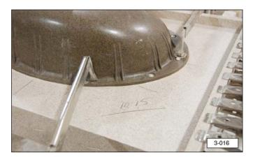
**Note**: Be very careful not to disturb the acrylic adhesive joints during the one hour cure time.
