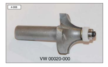
Before rounding the opening in the countertop, make sure the depth of the router bit is adjusted to allow the bearing to ride against the sink, just below the seam. Set the depth of the router bit to avoid cutting into the top surface of the countertop, causing an unsightly groove. To avoid damage to the sink and countertop, do not cut against the rotation of the router bit (from right to left), and do not allow the router bit bearing to travel into the sink drain overflow opening.
