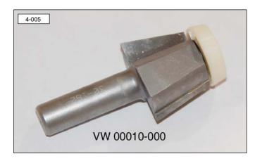
Before beveling the opening in the countertop, make sure the depth of the router bit is adjusted to allow the bearing to ride against the sink, just below the seam. To avoid damage to the sink and countertop, do not cut against the rotation of the router bit (from right to left), and do not allow the router bit bearing to travel into the sink drain overflow opening.
