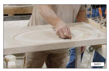
**Note**: Wear protective disposable gloves when working with the two-part acrylic adhesive. Remove excess acrylic adhesive with a flat blade putty knife. Clean up excessive acrylic adhesive with denatured alcohol and a clean cloth.
