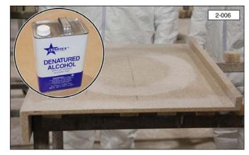
Before glue-up, wipe all the sanded surfaces with a clean cloth and denatured alcohol. Remove all dust and let the surfaces dry completely.
