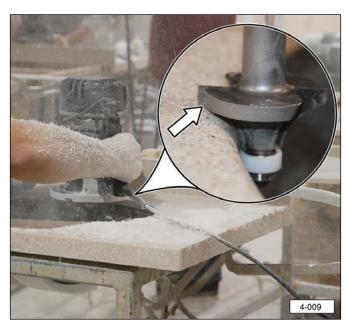
**Note**: Marks on the sink caused by the router bit bearing will be removed during the sanding process in a later section.
