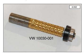
Before cutting the opening in the countertop, make sure the depth of the router bit is adjusted to allow the bearing to ride against the surface of the sink, just below the seam. To avoid damage to the sink and countertop, do not cut against the rotation of the router bit (from right to left) and do not allow the router bit bearing to travel into the sink drain overflow opening.
