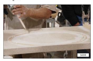
11. Use a spread stick to smooth out the adhesive. The adhesive should be just thick enough to hide the countertop surface underneath.
