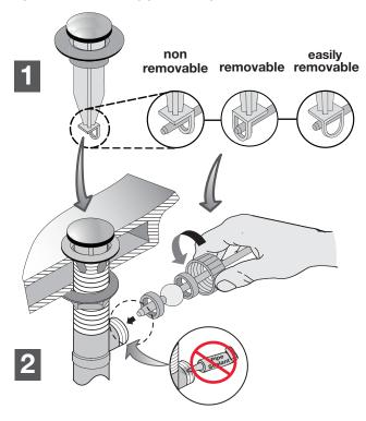
Step 7 Connect lift rod and adjust linkage
