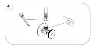
Apply teflon tape onto threads of water supplies.
