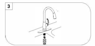
Secure the faucet to sink by installing plastic washer  $\cdot$  steel washer and nut onto it. Tighten with wrench.
