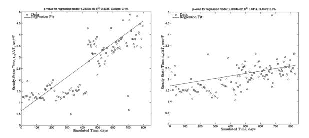
Figure 6.Regression Model Plots Time to steady state temperature for an untreated heater (Left) and NuvoH<sub>2</sub>O-treated heater (Right).
