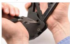
Tap the adjustment pin (#3) out as far as you can with needle nose pliers then remove pin by hand using a pulling/wiggling motion.
