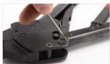
Remove existing E-Clip (#4) by prying it away from the pin with a flat head screw driver or needle nose pliers.
