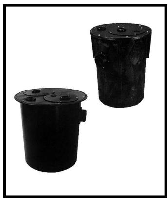
The corrosion resistant basins and covers are available in light weight, durable, simplex and duplex styles in basin diameters from 18" to 36". The basins include an inlet hub. The gas tight covers come complete with vent and discharge flanges, cord seals, gasketing and hardware. Access openings allow easy removal of pump without disturbing vent connection. Larger sizes and alternate configurations available as specials. Contact factory with particular application requirements.
