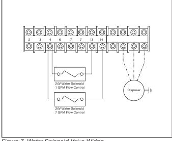
Figure 7. Water Solenoid Valve Wiring
