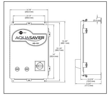
Figure 1. Control Center Dimensions
