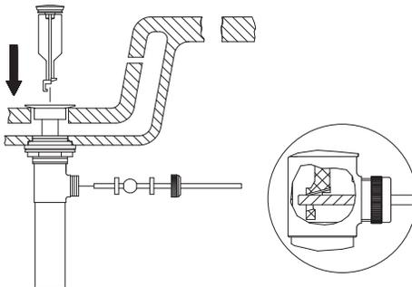
5. Insert stopper assembly (8) into drain. Insert ball rod (5) into rod port and into hole at bottom of stopper assembly.
