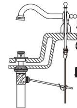
7. Insert bottom of lift rod (1) into hole at top of lift rod strap (3). Tighten with thumb screw (2).
