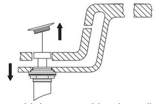
1. Remove old drain assembly. Clean all sink surfaces to remove old putty and dirt before installing new drain.
