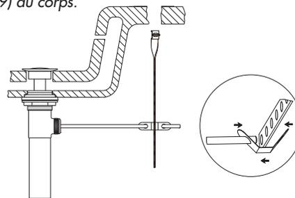
6. Place one end of spring clip (4) on end of ball rod (5). Pass the tip of the rod through the hole in the lift rod strap (3) and then through the hole on the other end of the spring clip (4).
