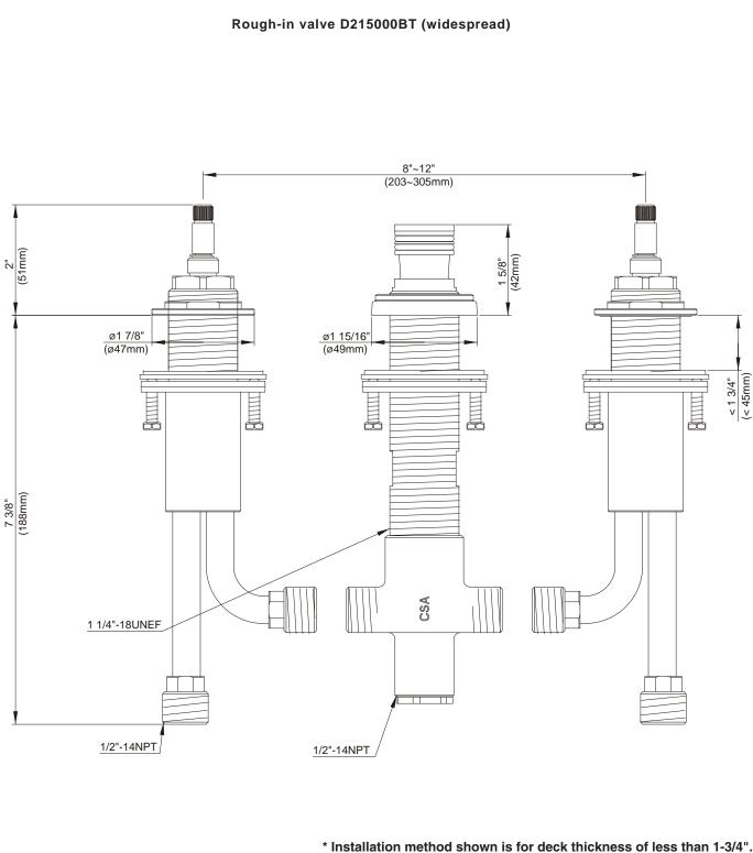
\* Installation method shown is for deck thickness of less than 1-3/4". If the installation is for deck thickness between 1-3/4" and 3-1/2", the sleeve nut needs to be reversed.
