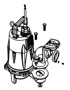
All the claws have a sealing grommet attached to it that provides the seal between the claw and base unit. This seal requires no maintenance. On GR30, GR22-LE, AND GR22-FL a gasket should be used between the claw and pump – the gasket and mounting hardware are provided with the pump. The stock flange that is shipped with the pump should be removed and replaced with the claw.
