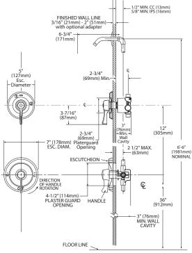
NOTE: This valve is not intended to be used as a shut-off valve. To prevent the potential of cross flow, check valves must be integral to the supply valve or installed in both hot and cold water supply lines. \*Refer to (ADAAG) guidelines or local codes for proper ADA installation.
