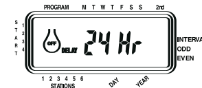
Figure 15: Display Showing Rain Delay
