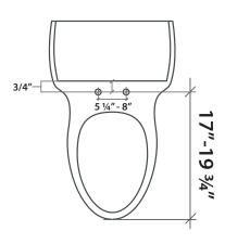
\* Note: the Swash Ecoseat 100 is designed to fit elongated toilets only, however this model will in fact fit select round fixtures. Please reference fit diagram for size verification. The Swash Ecoseat 100 will not fit French curve fixtures.
