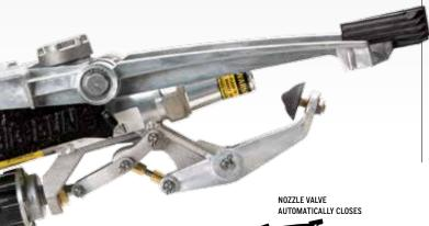
The SRNV100 is the standard SR100 Big Gun® configured with a simple mechanical valve which can be either hydraulically or electrically controlled and linked to the pivot control system. The nozzle valve improves end gun performance and efficiency by eliminating pressure loss, turbulence, and debris hang-up typical of other end gun control valves.
