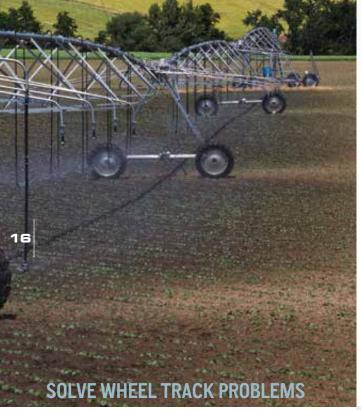
EXCESSIVE WATER IN THE WHEEL TRACKS CAN CAUSE SLIPPAGE OF THE TIRES, CAUSING THE SYSTEM TO SLOW DOWN IN WET AREAS AND STEEP SLOPES -INCREASING THE APPLICATION DEPTH IN RELATION TO OTHER PARTS OF THE FIELDS. DEEP WHEEL TRACK RUTS ARE ALSO DETRIMENTAL TO THE EQUIPMENT AND HARVESTING EFFICIENCY.
