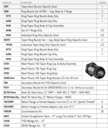
\*See 150/200 Flange Adapter to Female Adapter page 51. 3" FNPT (\*8403-001); 3.5" FNPT (\*6621-000); 3" BSP (\*6621-001); 4" (\*9127). Contact Factory for availability of anodized & power coated options.
