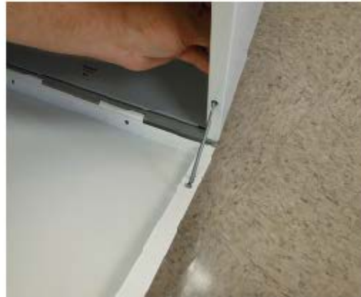
Step 3: Bring Door Forward and Place Screw head into Keyhole.
