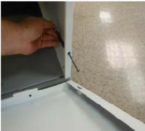
Step 2: Pushing From Backside of Spring Assembly - Push the Screw Head Thru the Hole in the Cabinet.
