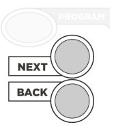
RAPID ADVANCE: While programming, holding down the UP or DOWN button will cause the flashing display value to rapidly advance. Rapid advance can also be used with the NEXT and BACK buttons to rapidly advance through zones.
