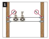
Determine stub out height. Secure top bracket to face of stud bay.
