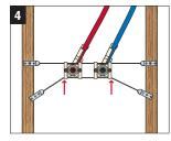
As close as possible to each block, bend the bottom bracket downward. Bending the bottom bracket provides the most rigid installation.
