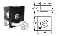
Allows outside fresh air for combustion through the wall thimble without having to cut a second hole into the wall. Comes with an insulation ring to reduce air infiltration where the pipe slips through the thimble. The 2" diameter flex hose is 10' in length. Clamps included. Can be used in US and Canada. Patented.
