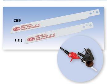
14 TPI (teeth per inch) work best on materials at least 1/8" thick. 8 TPI work best on materials at least 3/16" thick. Use fewer teeth per inch on softer materials like plastic.
