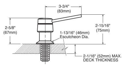
**NOTE:** DESIGNED TO BE INSTALLED THROUGH 1 HOLE 1-1/8" DIAMETER
