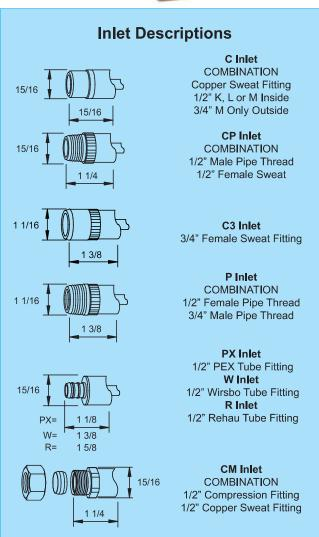
When ordering, specify model, inlet and wall thickness.
