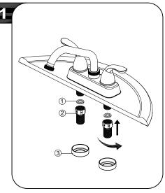
If installing onto a sink or countertop more than 1" thick, from underside, assemble washer (1), connector (2) and mounting bracket (3) onto body.
