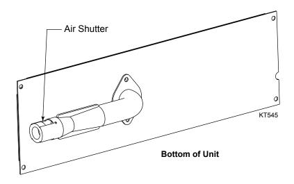
Figure 8 Adjust Air Shutter - 1/4" Open
