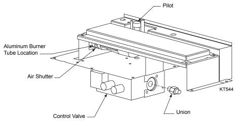
Figure 2 Remove Union from Control Valve (Millivolt Unit Shown)
