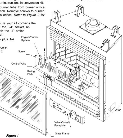
Remove Valve Cover/Faceplate, Engine/Burner System and Glass Frame (BDV Millivolt Unit Shown)
