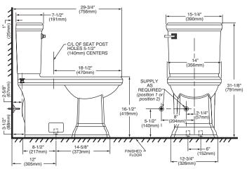
IMPORTANT: Water supply on the wall is required at 2-1/4" or 8" from centerline of the toilet (see rough-in). First suggested position is hidden behind the toilet. The geometry of the toilet gives space for this installation. The second suggested position is next to the toilet. Between these two positions, the space for the supply between wall and toilet is limited to 3-1/2". In this case, check your supply and hose dimensions. **NOTES:**
