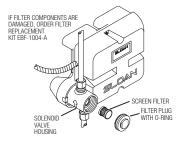
Clean the screen filter using fresh tap water only. If necessary, use a small brush to clean. Use caution while cleaning to prevent damage to the solenoid screen filter. If any filter components are damaged, order Filter Replacement Kit (EBF-1004-A).
