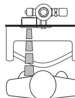
3. When the user steps away from the sensor, the loss of reflected light initiates an electrical "one-time" signal that energizes the solenoid operator, and activates the flushometer to flush the fixture. This occurs on the water closet approximately three (3) seconds after indication. This delay is built into the sensor to help prevent false flushing due to movement by the user. The circuit for both water closets and urinals then automatically resets and is ready for the next user.
