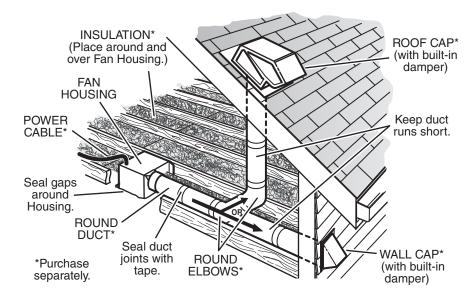
The ducting from this fan to the outside of the building has a strong effect on the air flow, noise and energy use of the fan. Use the shortest, straighest duct routing possible for best performance, and avoid installing the fan with smaller ducts than recommended. Insulation around the ducts can reduce energy loss and inhibit mold growth. Fans installed with existing ducts may not achieve their rated airflow.
