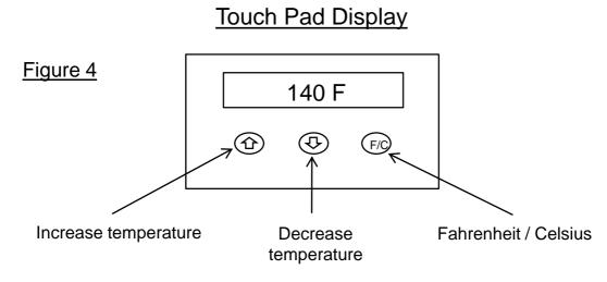
To trouble shoot the display board, shut off power to the unit. Press and hold all three buttons, and re-energize the unit. If display board is working properly, the word "Yes" will display. If the board has a fault it will display "No" and you should call technical support for a replacement.
