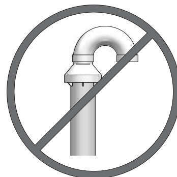
Figure 5-5 Do Not Install U-Bend to Rain Cap
