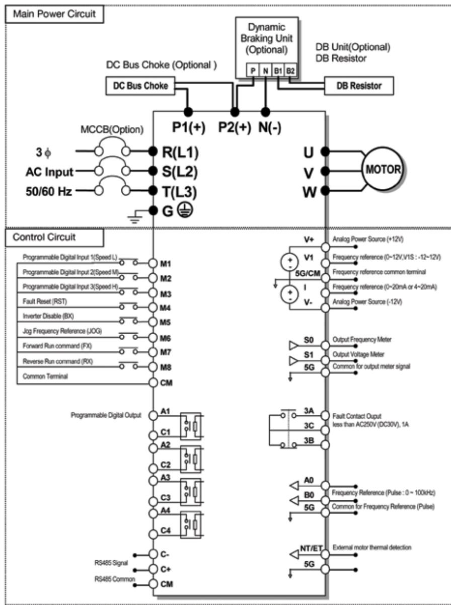
Note : 1) 5G is Common Ground for Analog Input/Output for 7.5-40HP
