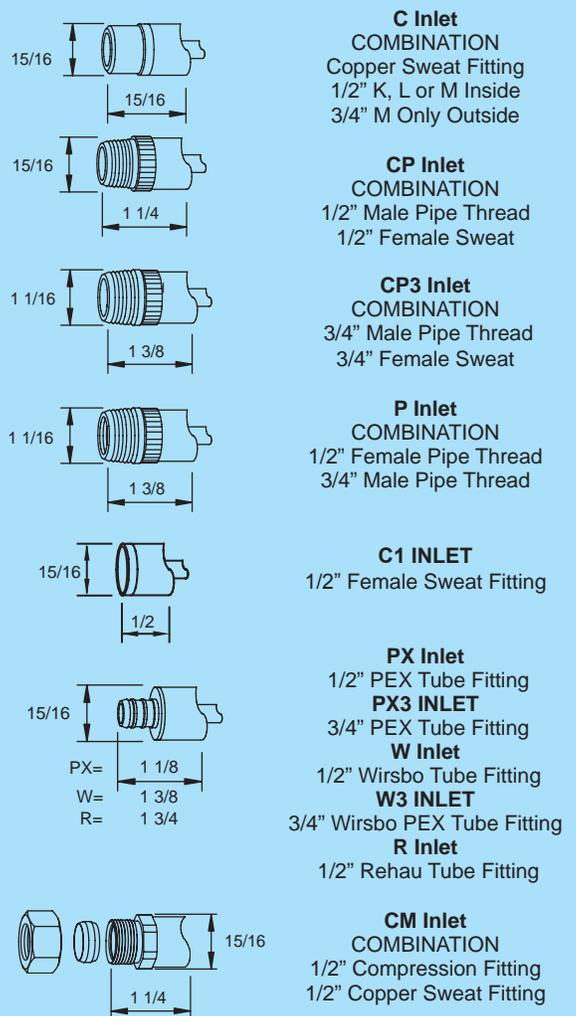
**When ordering, specify model, inlet and wall thickness.**
