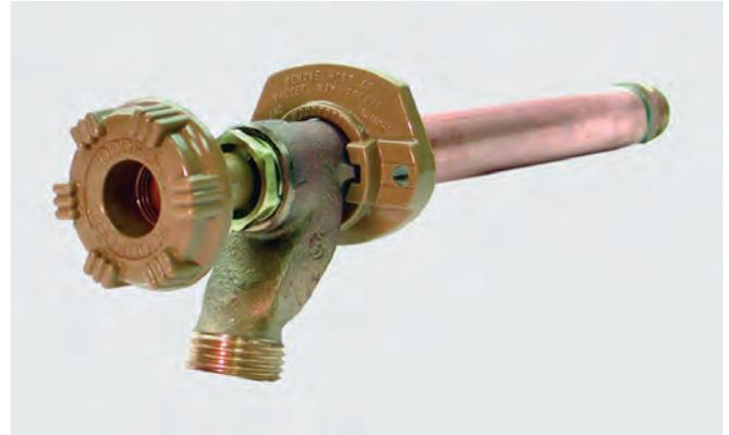
**WARNING** - Faucet must be installed with downward pitch toward nozzle and hose must be removed in freezing weather or faucet may freeze and burst.
