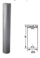
Use to reline masonry chimney with 0/0 clearance. Factory-insulated. Twist-lock fittings and pre-drilled hole (one screw required). UL Listed for zero clearance between masonry and combustibles, plus zero clearance between liner and masonry. 304 stainless steel inner and aluminized steel outer. Note: to calculate the installed length of 5", 6", and 8" DuraLiner pipe subtract 1 ½" from each joint overlap of liner pipe sections.
