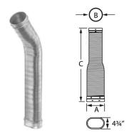
Use through damper and smoke shelf area. Use to connect from oval stove outlet to round DuraLiner. Use with DuraLiner ProMesh and ProFoil, where flex extends into clay liner, for zero-clearance applications. Built from 1-ply construction, .005" 304 stainless steel.
