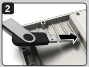
Insert USB drive into the controller USB slot.
