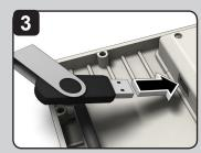
Insert USB drive into controller USB slot.
