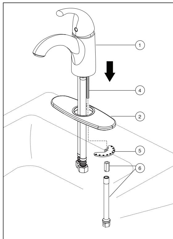
**SHUT OFF WATER SUPPLIES.** Position faucet (1) with single or three hole escutcheon (2) and baseplate (3) or gasket (3) on sink, studs (4) must pass through the holes on escutcheon (2) and baseplate (3). **Option:** If surface of sink is uneven, use silicone under the baseplate or gasket. Place metal bracket (5) over mounting stud (4) under sink. Secure with mounting nut & wrench (6).
