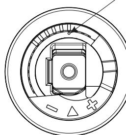
Indicator marks in minimum handle movement, minimum hot water flow
