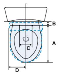
**Note:** Some styles of toilets may not allow the Washlet B150/B200 to be installed due to certain contours near the tank and bowl area (see figures below). In the figure on the left side below, dimension D not allow enough open space to accommodate the minimum width of 11 inches.
