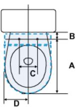
**Note:** Some styles of toilets may not allow the Washlet C200 to be installed due to certain contours near the tank and bowl area (see figures below). In the figure on the left side below, dimension D not allow enough open space to accommodate the minimum width of 9 inches.
