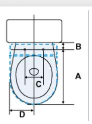
**Note:** Some styles of toilets may not allow the Washlet S300e/S350e to be installed due to certain contours near the tank and bowl area (see figures below). In the figure on the left side below, dimension D not allow enough open space to accommodate the minimum width of 9 inches.
