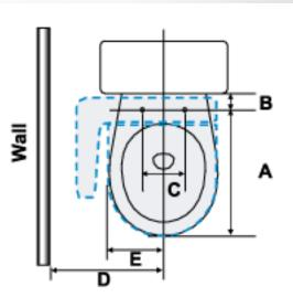
**Note:** Some styles of toilets may not allow the Washlet C100 to be installed due to certain contours near the tank and bowl area (see figures below). In the figure on the left side below, dimension D not allow enough open space to accommodate the minimum width of 11 inches.
