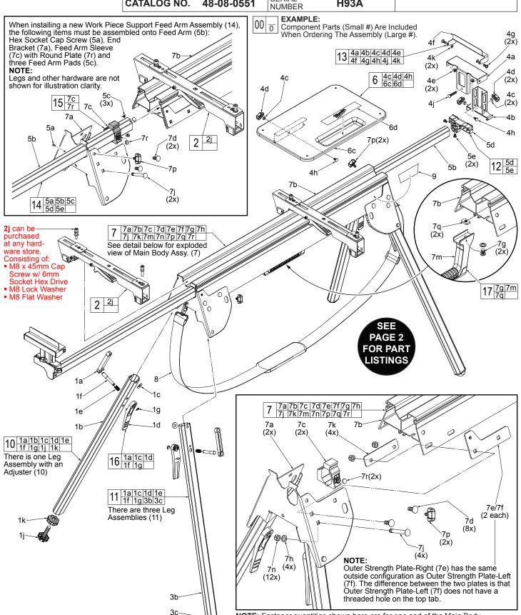
MILWAUKEE ELECTRIC TOOL CORPORATION 13135 W. LISBON RD., BROOKFIELD, WI 53005 **NOTE:** Fastener quantities shown here are for one end of the Main Body. For illustration clarity, only one corner (leg area) is depicted.
